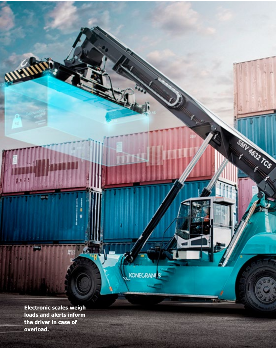
Front and roof windshield grids protect the driver from falling objects.
