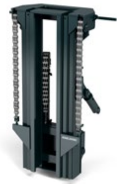
TRIPLEX, 3-STAGE WITH FREELIFT specific for very low-ceiling warehouses.
