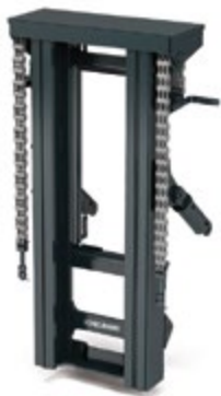
DUPLEX, 2-STAGE, NO FREELIFT (standard)
