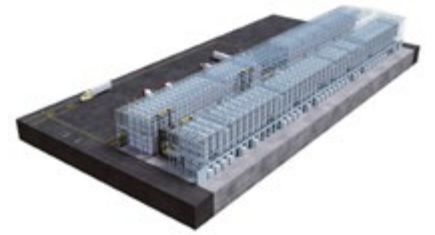
AUTOMATED HIGH-BAY CONTAINER STORAGE (AHBCS)
