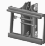
Carriage sideshift / fork positioning
