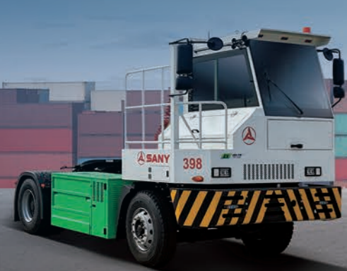
Plug-in Electric Terminal Tractor SM2500
